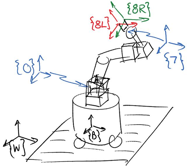
Determine the full forward kinematic model from the World frame to the fingertips.
