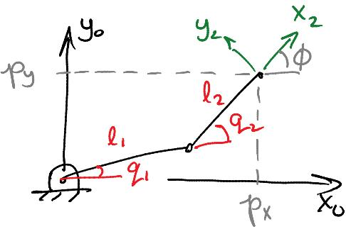
$$q \Rightarrow T_2(q) = \begin{bmatrix} s_\phi & c_\phi & p_y \\ 0 & 0 & 1 \end{bmatrix}$$
