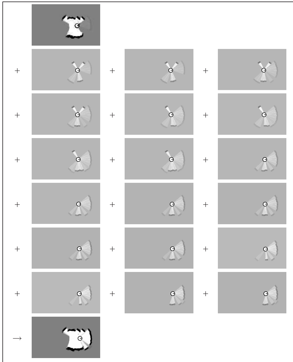
Figure 2.6: Incremental mapping in a corridor environment. The upper left image shows the initial map and the lower one contains the resulting map. The maps in between are the local maps built from the individual ultrasound scans perceived by the robot.
