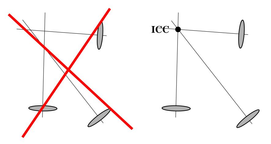
For rolling motion to occur, each wheel has to move along its y-axis
