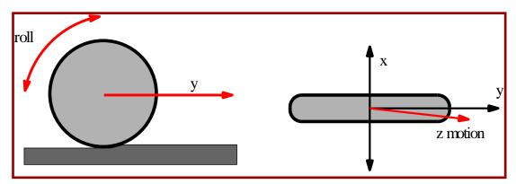
we also allow wheels to rotate around the z axis
