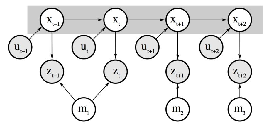
Landmark variables are all disconnected (i.e. independent) given the robot's path
