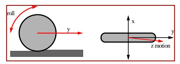
we also allow wheels to rotate around the z axis
