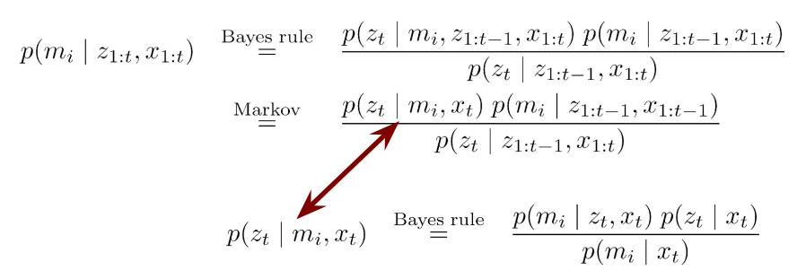
Defining a forward sensor model conditioned on only one cell is impossible, therefore, we use Bayes rule again to apply an (heuristic) inverse sensor model.
