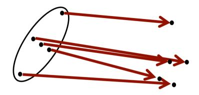
Transform each sigma point through the non-linear function
