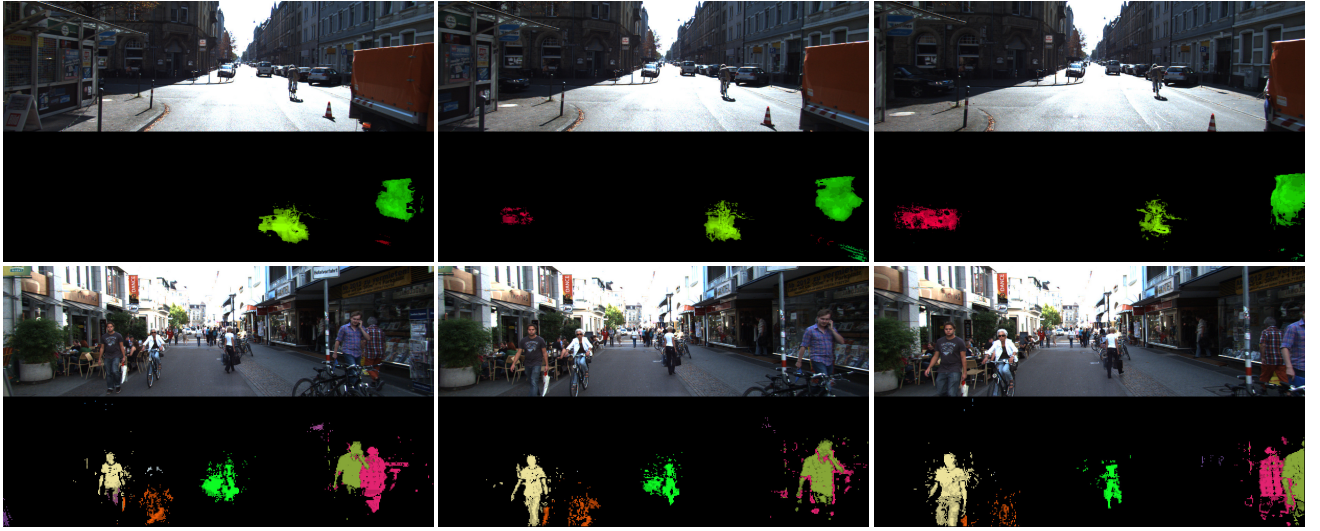
Fig. 4: Examples of temporal coherent label output of the proposed method. Top row shows the immediate detection of a car as it enters the scene denoted by the red cluster introduced in the middle frame. The bottom row demonstrates correct label assignments are maintained over multiple frames, even during temporary occlusion of the pedestrian on the right of the image.
