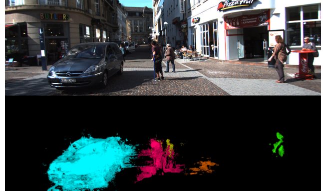
Fig. 1: Example detection of multiple dynamic objects discovered using our proposed method that corresponds to the input image sequence shown above. The different colours (hue) in the output image represents the multiple object instances detected, while the intensity denotes the likelihood of the assigned class at each pixel. These objects were detected using only the motion of the scene and not any off-line models describing the visual appearance of the objects.
