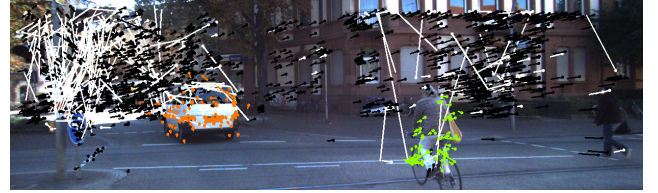
Fig. 3: Sparse optical flow vectors grouped by motion. Static points are shown in black, while the dynamic points are coloured by their cluster assignment. Points with low density in motion space (considered noise) are marked in white.
