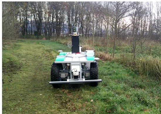
Fig. 1. Our robot navigating autonomous in a forest environment. We need to cope with grass of various heights, small trees and bushes. The corresponding point clouds need to be dealt with differently depending on the type of terrain the robot moves on.
